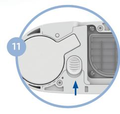
Insert column into the Inogen One® G3 concentrator. Do not leave the column exposed; it should be inserted into the Inogen One® G3 as soon as the dust caps have been removed.
