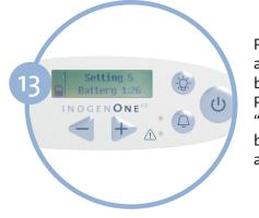
Press and hold the light button for 10 seconds and screen will display "sieve reset". Release button once message is displayed on screen. Press the bell button once and screen will display "sieve reset successful". Press the power button to turn on the Inogen One® G3, and use normally.
