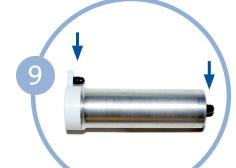
For the column installation, remove dust caps of new column. Make sure there is no dust or debris where the dust caps were located.
