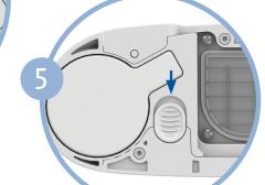
Remove column by pressing the latch button with thumb or finger.
